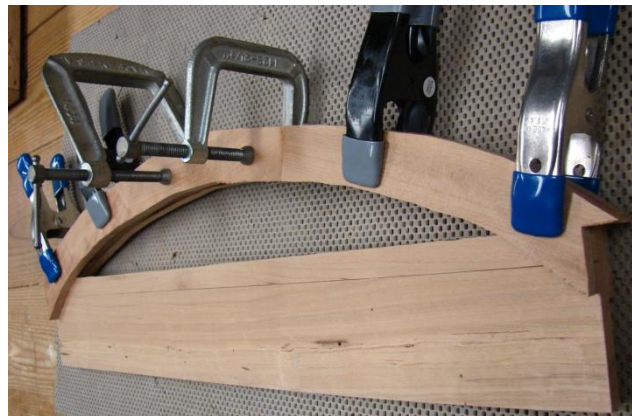
Figure 3 Wood strips are glued up to a thickness just greater than the desired rope diameter.
