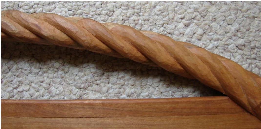
Figure 5 Carved rope handle for a tool box in cherry with a Tung oil finish.
