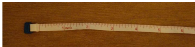
Figure 4 A coated fiber tape measure is flexible enough to follow the curve of the rope and rigid enough to draw the line that connects the dots.
