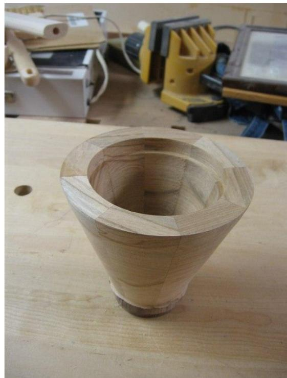
Figure 7 The stave assembly following preliminary turning. A rabbit was added to enable turning of the opposite end of the assembly.
