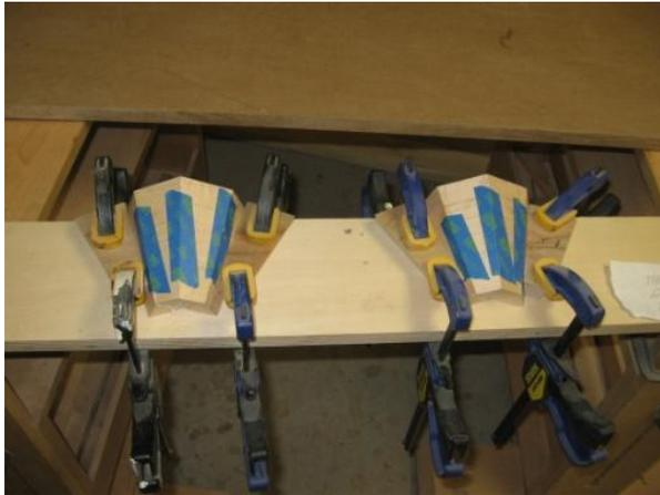
**Figure 4** Glue up of halves using cauls
