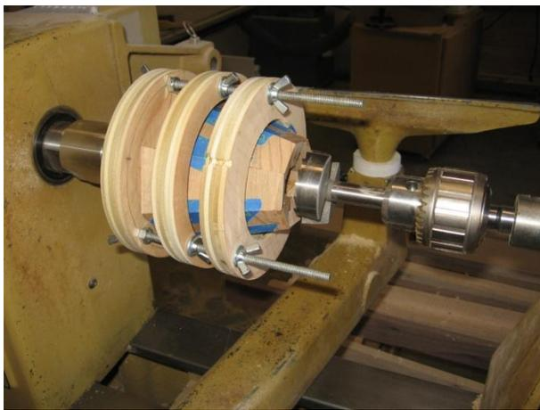
Figure 6 Clamping mechanism with stave assembly inclosed
