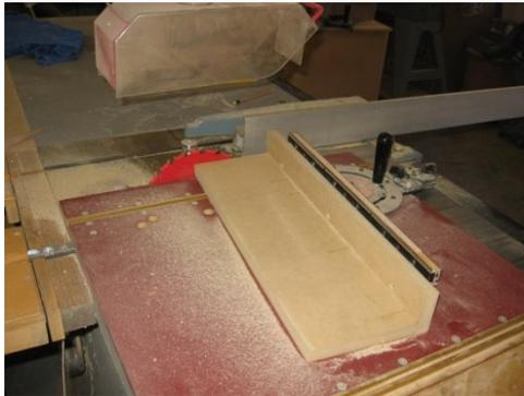
**Figure 1** Incra sled with Aux fence. Note saw fence used as stop.
