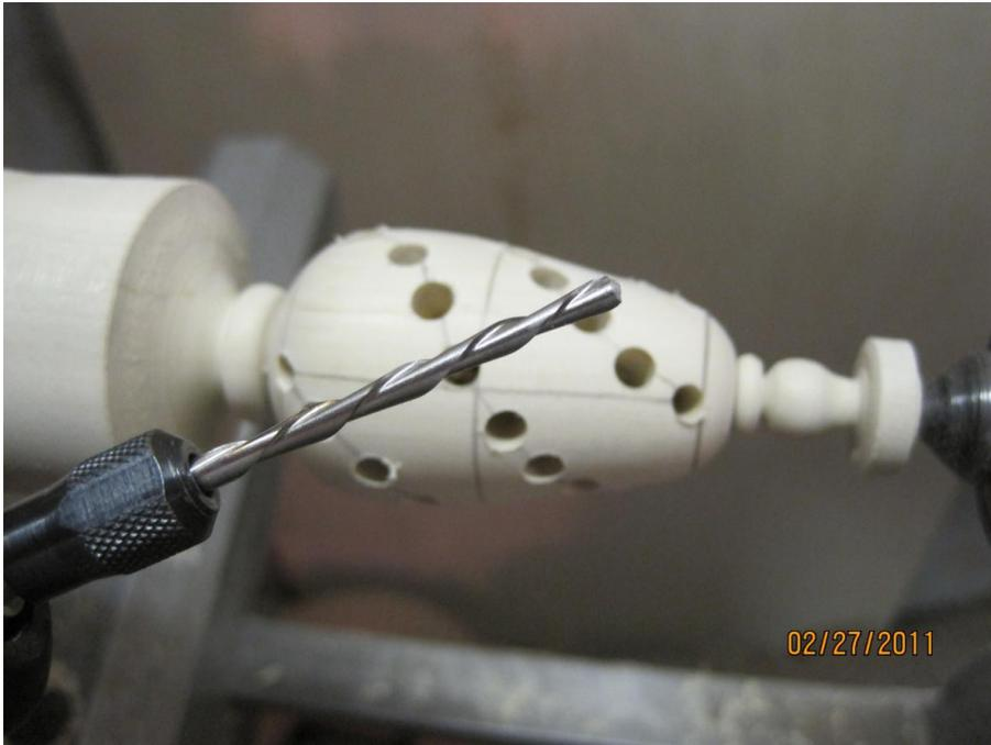
The next thing I do is to route a shallow trough connecting the holes. Here is a close-up of the bit I use in a Dremel tool. It looks like a Roto-Zip bit, I'm not sure, but it was included with the Dremel. A 1/8" drill bit could also be used. The reason for the trough is to help prevent the bit from jumping out and skating across the surface. I hold the Dremel on a low angle and gently route a channel from hole to hole.
