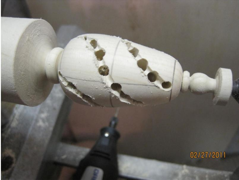
Here, the shallow channels are completed and I'm ready to open things up between the holes using the same Roto-zip type bit. This bit cuts aggressively, so a light touch is best.
