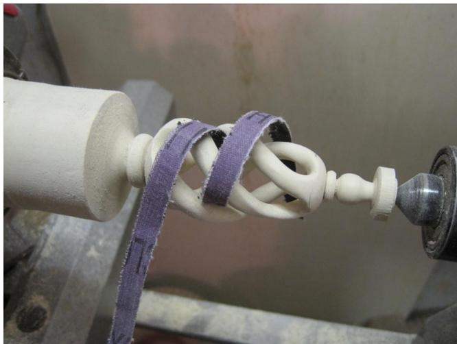
Sanding has begun starting with 80 grit cloth backed sanding strips. I tear the strips to about 1/4" or 3/8" in width. Continue through the grits removing scratches from the previous grit.
