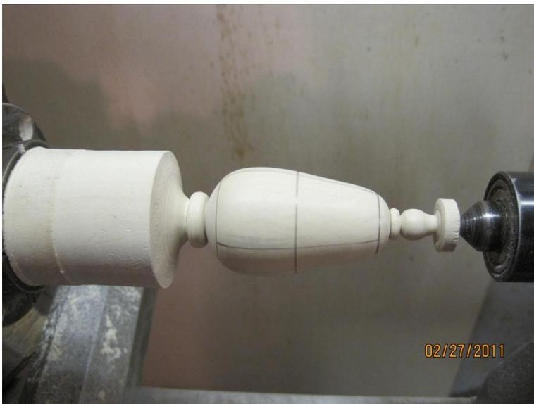
The layout consists of four evenly spaced horizontal lines called start lines. The index feature on most lathes makes this easy. The three vertical lines are pitch lines. These are easily done with the lathe running. On this example, the spokes, or bines as they are called, will make a  $\frac{1}{2}$  twist, This means when looking at the completed finial a bine will start at the bottom and stop half way around from where it began. You could also
