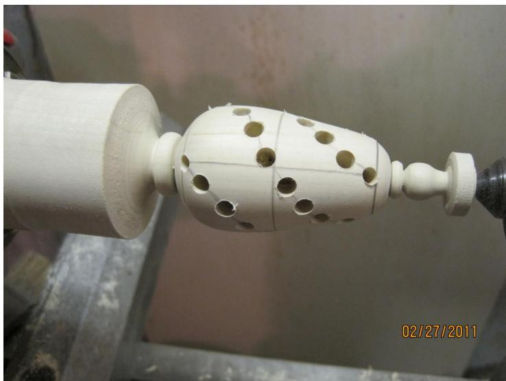
Using brad point bits, I have drilled holes on the cut lines. It's important that each hole be drilled toward the center of the piece. I used a 4mm bit for the four holes at the top
