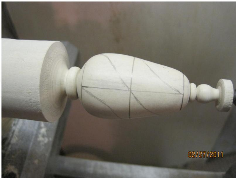
Here is where a decision needs to be made. Do you want a right or left hand twist? For this example I chose a right hand twist, but being a southpaw, a left hand is easier for me. Using a pencil I have started at the intersection of a pitch line and start line and draw diagonally to the next start/pitch line intersection. These are called the cut lines. At this time, for safety sake, you should unplug the lathe. It will be used for holding the piece in a still position only.
