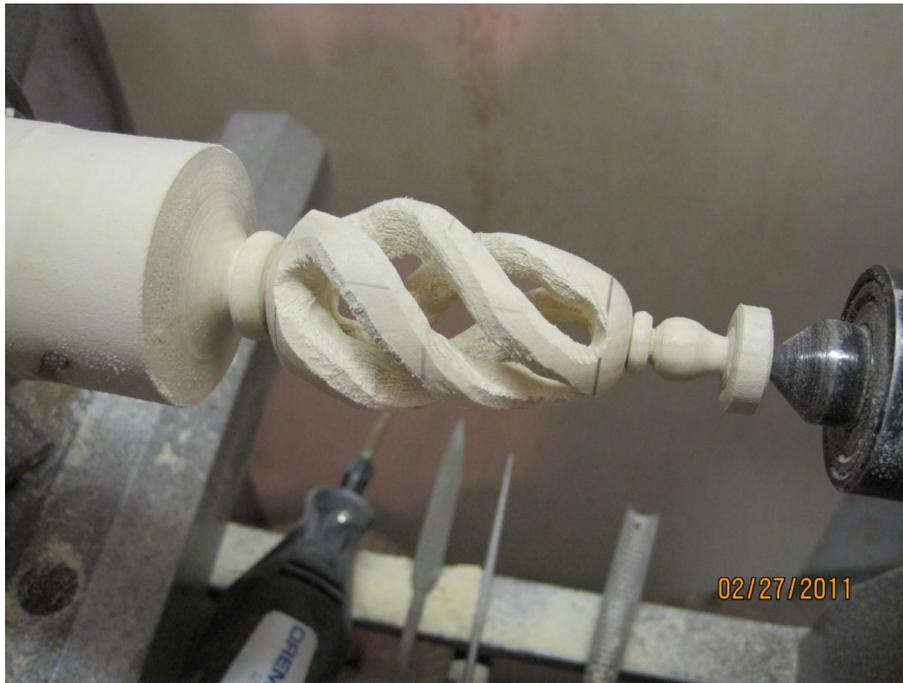
The bines are starting to take shape and almost ready for sanding, but not yet. You want to be careful to keep the bines equal in size. The tools used can be seen (although blurry) sitting on the lathe bed.
