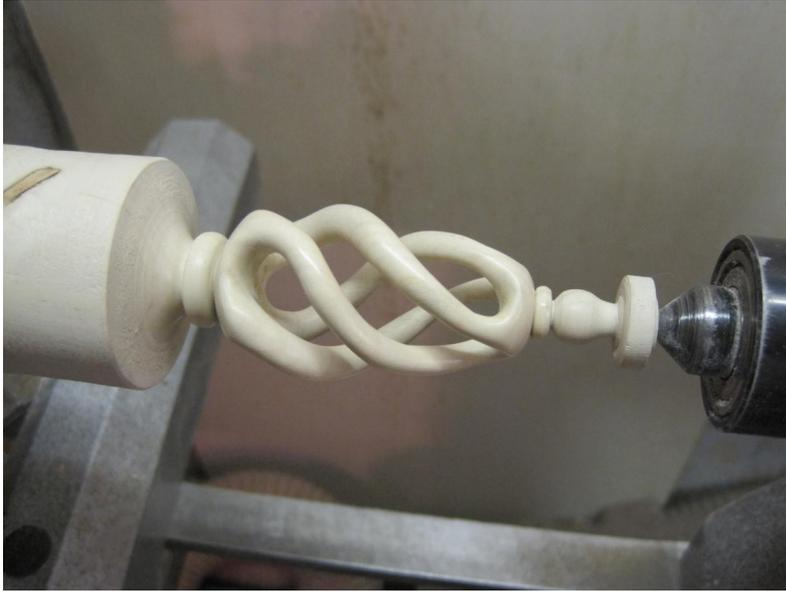
The sanding is finished. On this piece I sanded to 1200 grit, then I buffed each bine with 2,000 and 4,000 grit Abralon.
