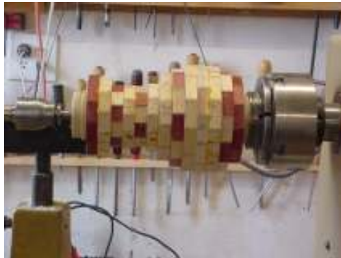
Figure 5. Segmented Vessel ready for shaping.
