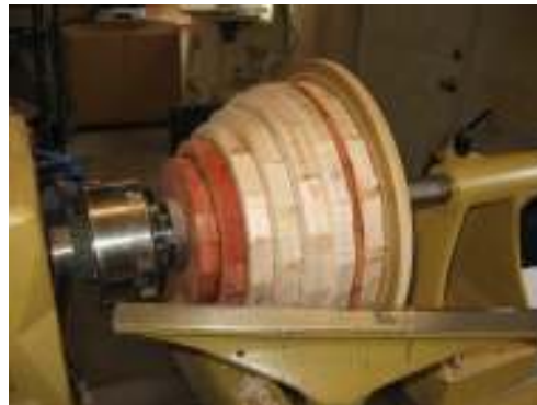
Figure 4a. Aligning rings on the lathe.
