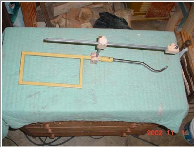
View of handle assembly with laser attachment mounted. The laser is in the block to the far right above the point of the cutting tool. All standard 3/4" cutting tools will mount in the handle assembly. The laser assembly is adjustable in three axes to let the turner place its spot exactly where it is needed to be relative to the cutting tool edge.
