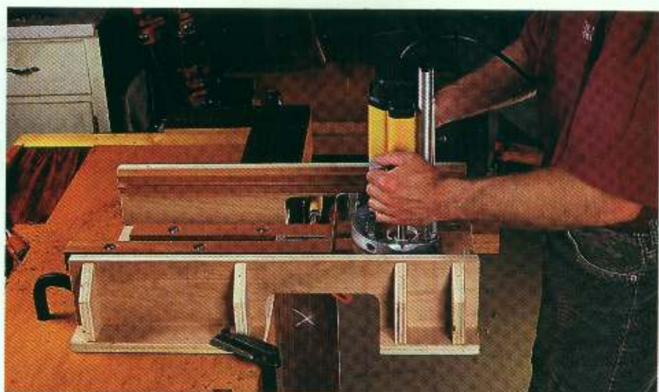
End cutting. Rout a mortise for a loose tenon by clamping the stock vertically.
